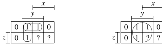
(a) Grouped without don't care state. (b) Grouped with don't care state.
