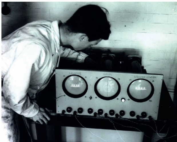
Figure 4.11 Sid Barton with 9-inch tubes which implemented the EDSAC operator display. (Copyright Computer Laboratory, University of Cambridge. Reproduced by permission under the Creative Commons Attribution Licence, photographer: Unknown, source: http://www.cl.cam.ac.uk/Relics/jpegs/edsac99.35.jpg )
